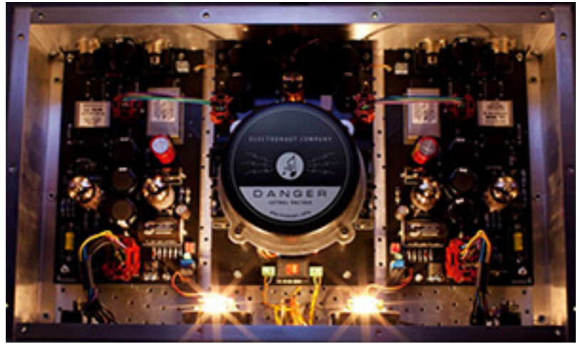
Lundahl transformers inside an Electronaut mic/instrument preamp.
