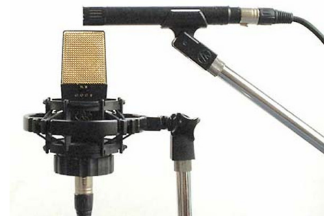
Figure 3: Two popular microphones placed in a mid-side (MS) configuration.
